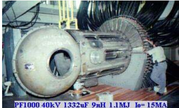
Figure 4b. 1 MJ PF1000 plasma focus
