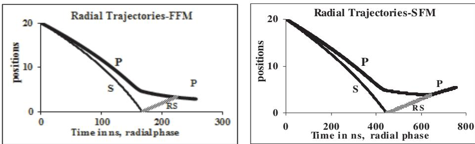
Fig. 6. The FFM (left) produces a much tighter pinch (pinch radius ratio of 0.15a) than the SFM (right) with a pinch radius ratio more than twice that of the FFM.
